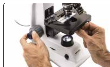
Regulation of diaphragm aperture
